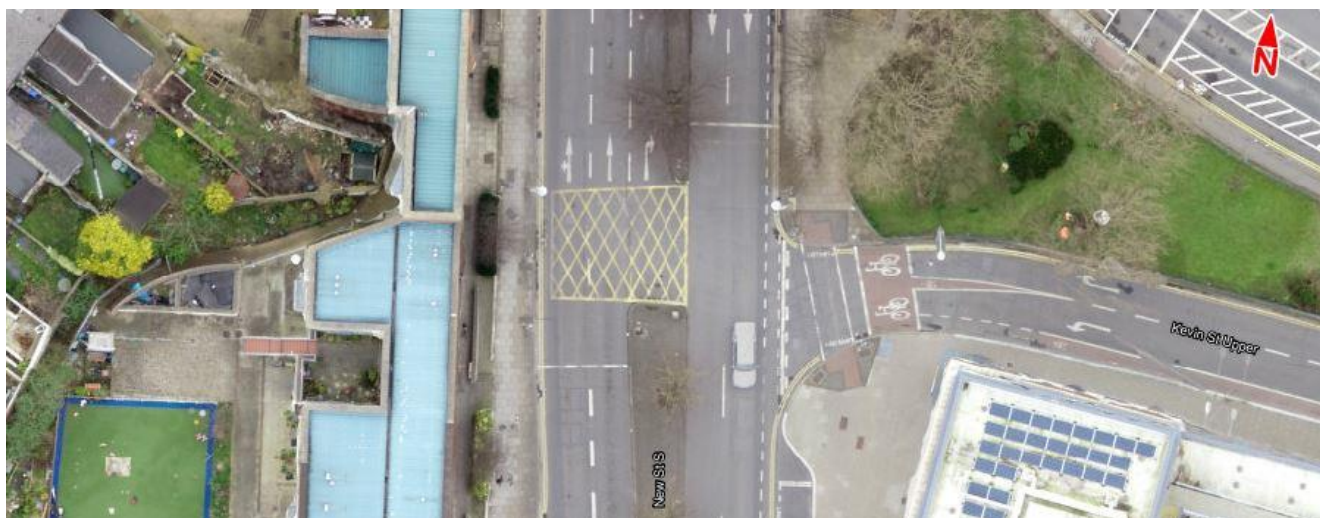
Image 6.11: R137 New Street South / R110 Kevin Street Upper (south) Three-Arm Signalised Junction
